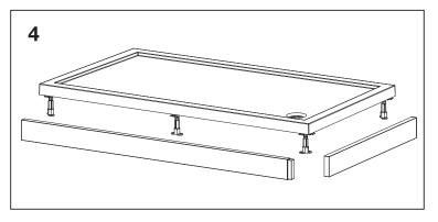
**4**. Cut the panels to required size and push the cover panel into place using the panel clips under the lip of the tray to secure.
