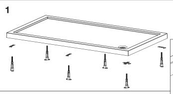
1. Fix the legs and panel clips to the base of the tray by screwing the leg through the clip and into the inserts (which are installed into the base of the tray as standard) to give an evenly supported structure.
