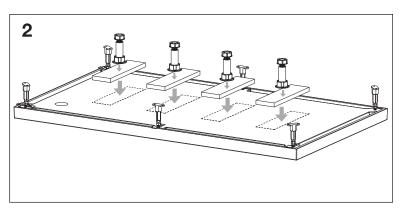
2. Evenly distribute the wood blocks along the centre of the base and silicone in place. Leave to set following the manufacturer's guidelines.
